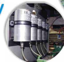
The Electro-Mechanical Lubrication Unit
